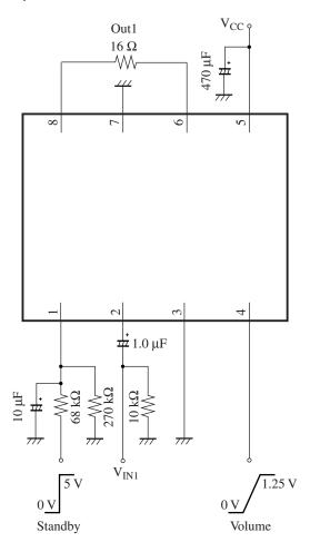
Note) The IC is on standby if the STB pin is open.
